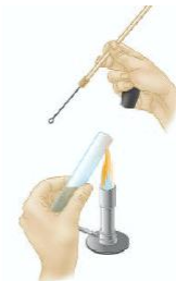
(c) Remove the cap, and flame the opening of the tube. Do not place the cap down on the table.
